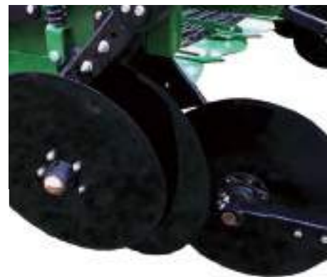
Parallel link arm on third coulter
